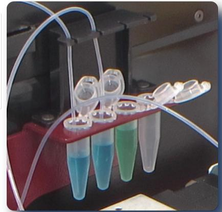
Automatic fluid handling allows for collecting and saving a sample. Flowrate can be adjusted across a large range using a syringe pump.
